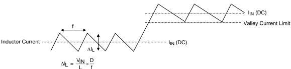
Figure 5. Inductor Currents In Current Limit Operation
