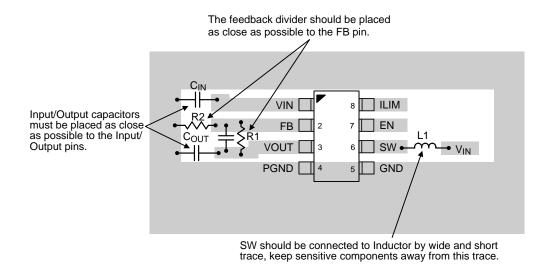
Figure 7. PCB Layout Guide
