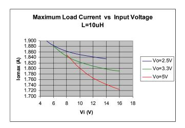
Figure 2. Theoretical maximum load current curves
