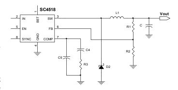
Figure 3. Compensation network provides 2 poles and 1
